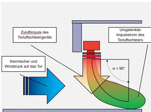
**Picture 1: Shielding force of an air curtain, due to the impulse change by the air curtain. Schematic view**
