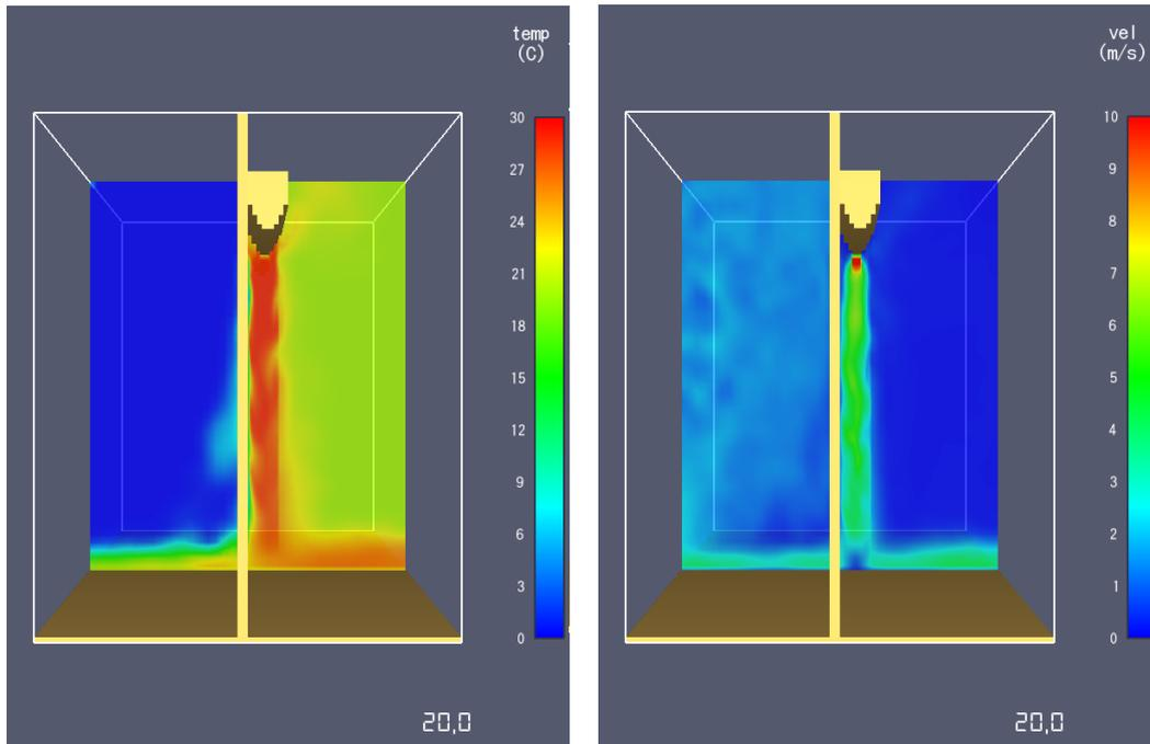
**Picture 7: Temperature field (left) and velocity field (right) on the axis of the room, with the door air curtain switched on, with only one homogeneous stream (single), after 20 seconds**
