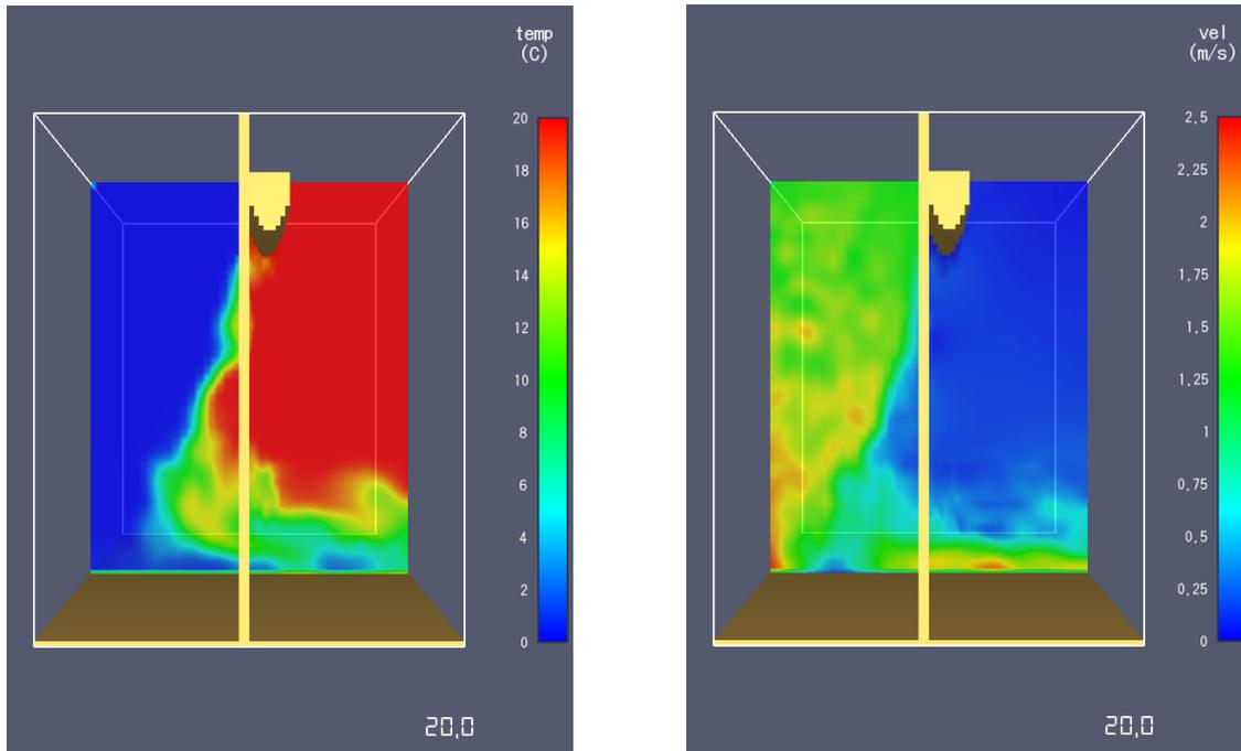
**Picture 6: Temperature field (left) and air velocity field (right) on the room axis, with the air curtain missing or deactivated, after 20 seconds.**
