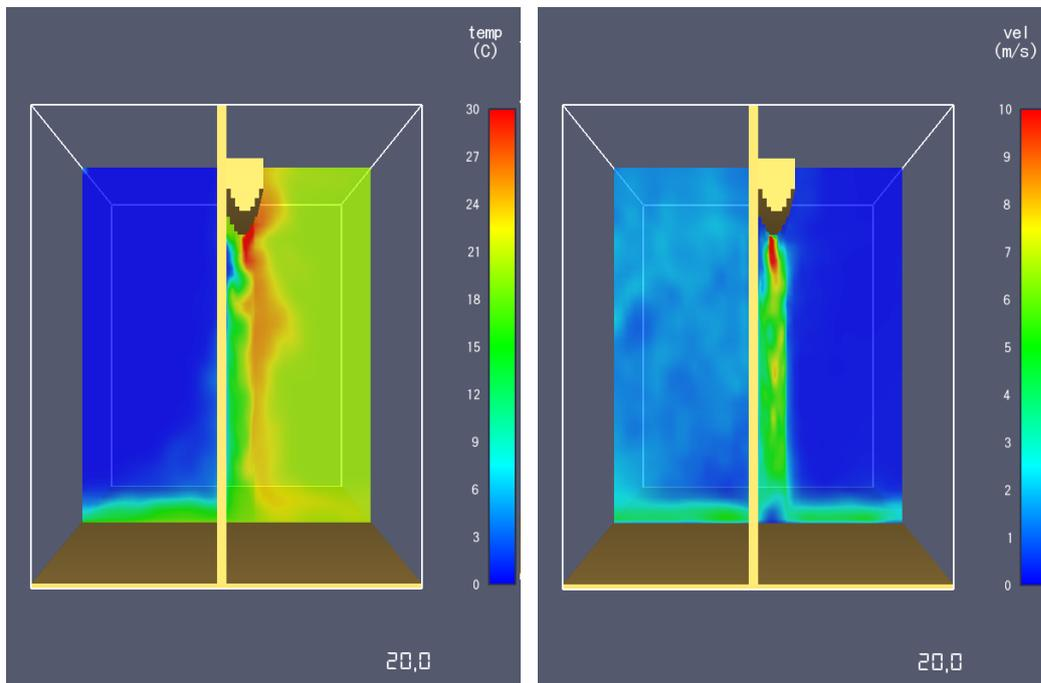
**Picture 8: Temperature field (left) and velocity field (right) on the room axis, with the door air curtain switched on: ProtecTor**
