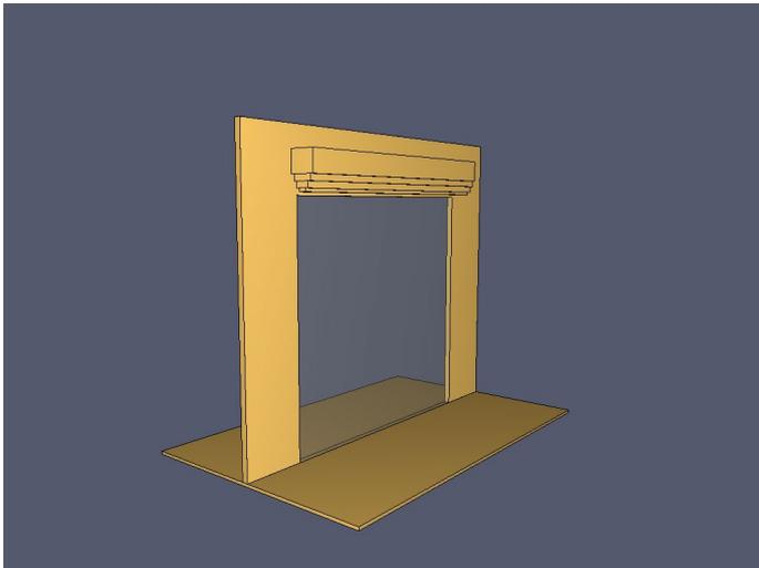
Picture 4 shows the geometry of the case file. A ProtecTor system has been installed right above a 4 m wide and 5 m high door opening.
