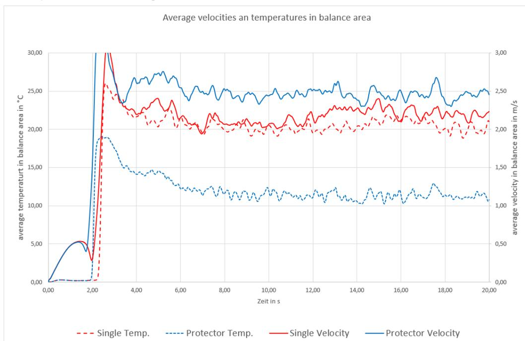
**Diagram 1: Depiction of the averaged measured values in the balance area, over the entire calculation time.**
