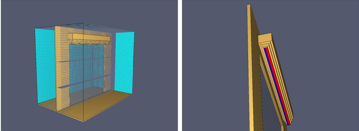
**Picture 5: Discretisation of the flow area (left), distribution of the outlet openings (right)**
