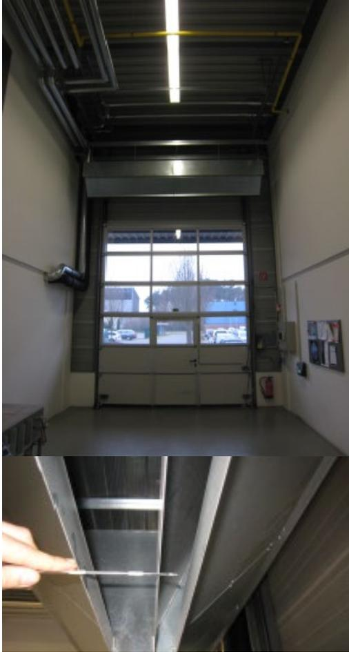
In the Kampmann R & D Center, a standard ProtecTor device was installed and measured. For this test not the thermal shielding effect was the focus of the investigation, but the determination of the leaving air velocities in the two air jets of the system.
