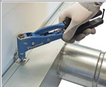
Fig. 6: Connecting the bracket to the housing
